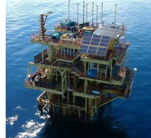
Solar PV and wind turbine systems are used on some of North Sabah's remote platform jackets
